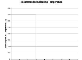
The soldering iron tip temperature should be set at 350°C (+10°C maximum) with the soldering duration not to exceed more than 3 seconds.
