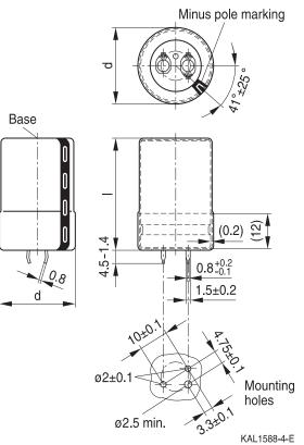
Snap-in terminals, length (6.3 + 1/-1.4) mm. Also available in a shorter version with a length of (4.5 - 1.4) mm. PET insulation cap is positioned under the insulation sleeve. Safety vent on the base.
