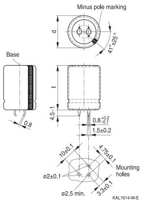
Snap-in terminals, length  $(6.3 \pm 1)$  mm. Also available in a shorter version with a length of (4.5 - 1) mm. PET insulation is marked with "PET" on the sleeve. Safety vent on the base.
