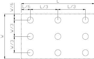
Lmax: The measured Maximum luminance of all measurement position. Lmin: The measured Minimum luminance of all measurement position. Note 7: Definition of Luminance: Measure the luminance of white state at center point.
